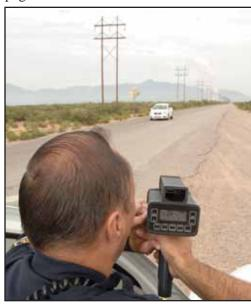
he had received a distance and speed reading from the laser gun. The operator would operate all laser guns in their "single shot" modes as is standard operating procedure as outlined in law enforcement training programs. If he did not receive a distance and speed reading, he would report it to SML staff recording the results. If the laser reported a distance and speed, this information was recorded. The tem-
